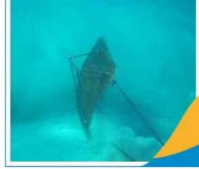
An Otter board dragged over the seabed presents a significant risk to offshore power cables when such a cable would not be buried sufficiently deep.
